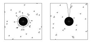
Figure 3-1– Crack induced by circumferential stresses
