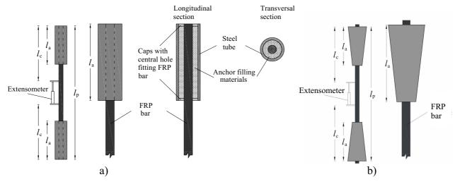
**Figure 6-1** – Examples of anchorage devices: a) by using steel tubes; b) by making cone ends of bar.
