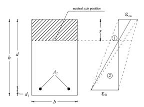
Figure 4-1 – Failure modes of FRP reinforced concrete section.
